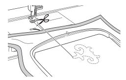
Using a hand sewing needle such as a ribbon embroidering needle, pull the bobbin thread to the top (wrong side) of the fabric, and then tie the upper thread and the bobbin thread together.
