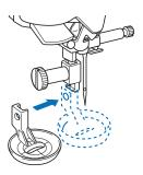
Tighten the screw with the included screwdriver.
