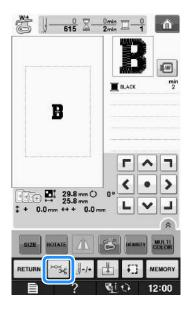
Press \_ to weaken the upper thread tension. (The tension number will decrease.)
