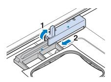
Insert a wound bobbin into the machine. (see "Setting the Bobbin" of "Basic operations".)
