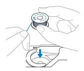
If the bobbin is inserted with the thread unwinding in the wrong direction, sewing will be done with an incorrect thread tension.
