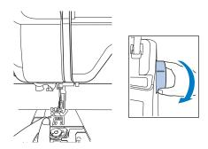
Gently pull the upper thread to bring the bobbin thread up through the needle plate.
