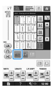
→ The key appears as , the quilting foot is raised to the necessary height, and then the feed dogs are lowered for free motion sewing.
