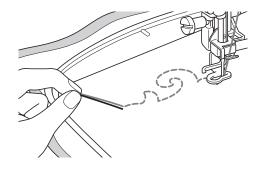
Stop the machine, and then tie the upper thread and the bobbin thread together to secure the threads.
