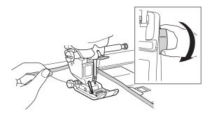
→ A loop of the bobbin thread comes out through the hole in the fabric.
