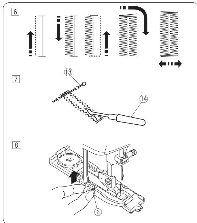
⑥ The buttonhole is sewn in the sequence as shown. When the buttonhole is finished, the machine will stop automatically with the needle in the up position.
