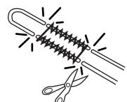
1 Use the same procedure as the square buttonhole sewing. Set the stitch width to match the thickness of the cord used.
