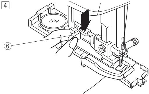
④ Lower the presser foot and pull the buttonhole lever down as far as it will go.
