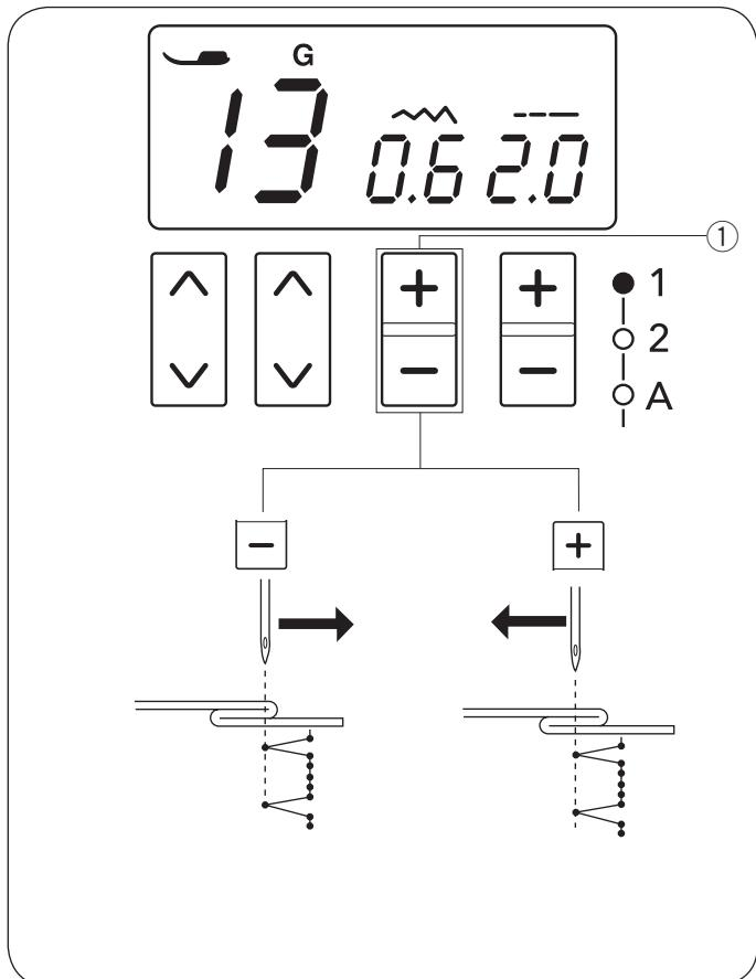
Adjust the needle drop position as follows:
