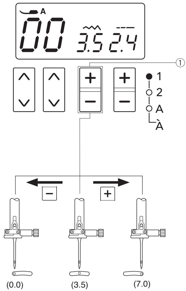
Press the “-” sign on the stitch width adjusting key to move the needle to the left.
