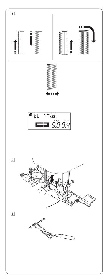
6 The buttonhole is sewn automatically in the sequence shown. When the buttonhole is finished, the machine will stop automatically with the needle in the up position.
