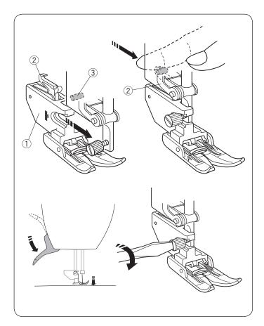
Attaching the Dual feed foot AD Attach the dual feed holder to the presser bar.
