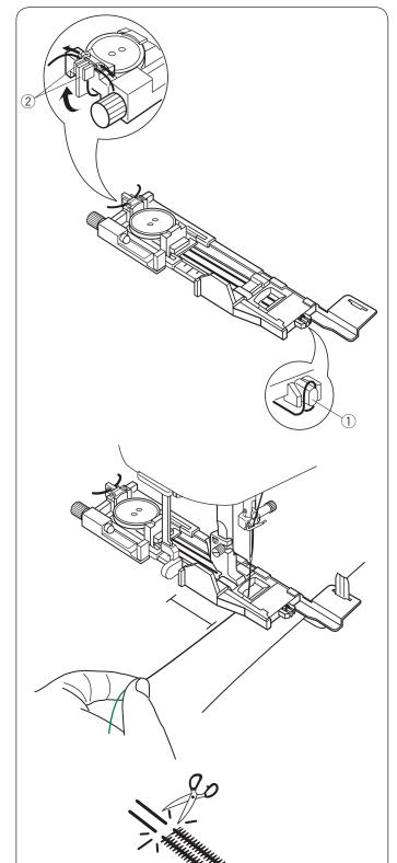
Place the button on the button holder on the buttonhole foot.
