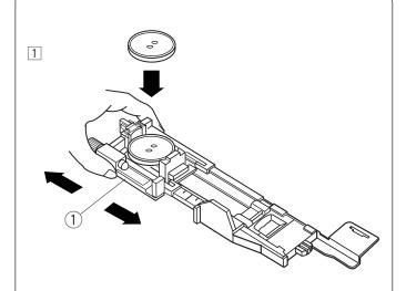
The size of a buttonhole is automatically set by placing a button in the rear of automatic buttonhole foot R.
