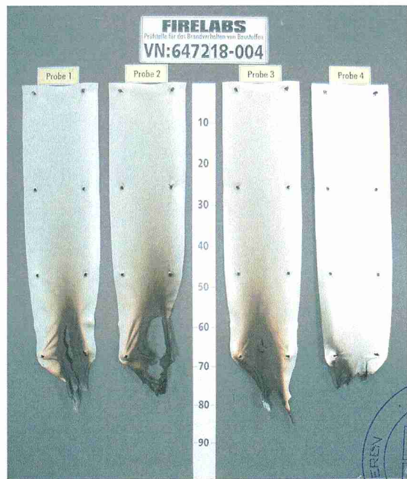
fig. 8 Photo of the test specimen after the test (sample 4: rear side)
