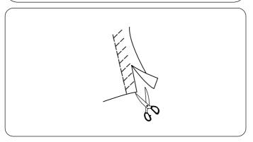
Place your fabric to allow a  $5/8^{\prime\prime}$  (1.5 cm) seam. Trim excess close to stitching. Be careful not to cut the stitches.
