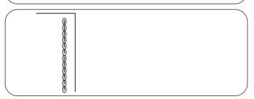
This strong, durable stitch is recommended when both elasticity and strength are necessary in order to insure comfort and durability. Use it to reinforce areas such as crotch and armhole seams. Also use for extra reinforcement when constructing items such as backpacks.
