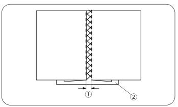
Use this stitch to join two pieces of fabric to create an open work appearance and add design interest. Fold under each fabric edge 5/8" (1.5 cm) and press. Pin the two edges to paper or tear backing 1/8" (0.3-0.4 cm) apart. Sew slowly, guiding the fabric so the needle catches the folded edge on each side.
