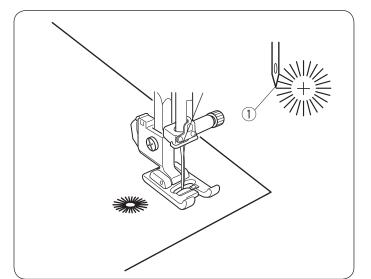
The eyelet is used for belt holes etc.
