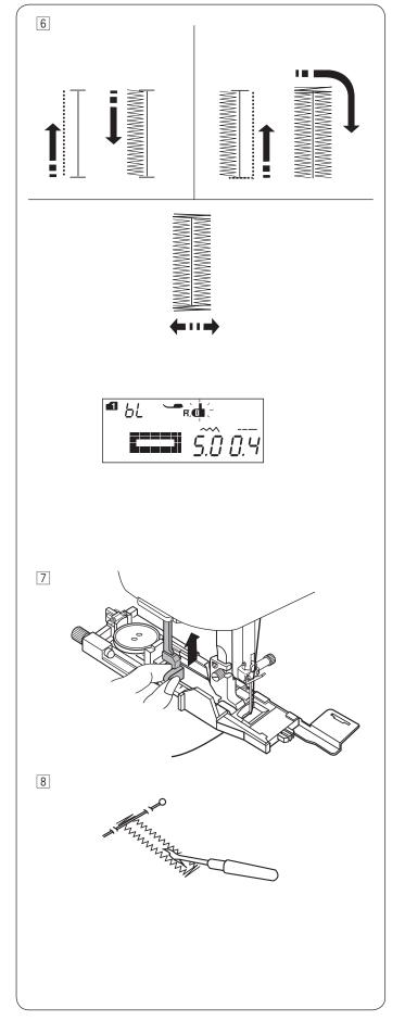
6 The buttonhole is sewn automatically in the sequence shown. When the buttonhole is finished, the machine will stop automatically with the needle in the up position.
