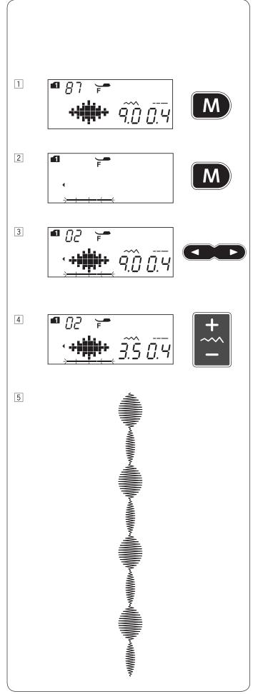
Individual Stitch Adjustment The stitch width and length can be individually adjusted for each pattern in a programmed combination. Example: Changing the stitch width of the one pattern in the combination
