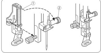
Attaching the Dual feed foot AD Attach the dual feed holder to the presser bar. ① Dual feed holder
