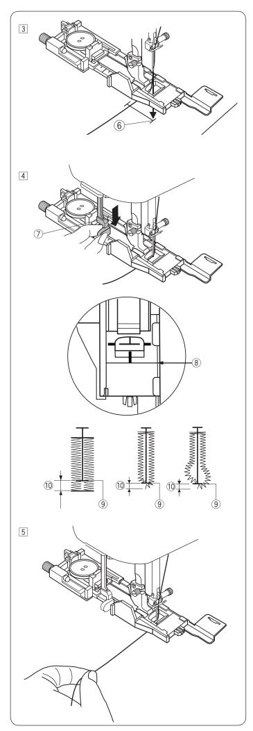
3 Draw the needle thread to the left through the hole of foot.
