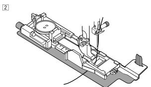
3 Place the fabric between the buttonhole foot and stabilizer plate. Lower the needle into the starting point by turning the hand wheel.
