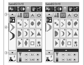
To delete a pattern in the middle of a combination, press the cursor key to select the pattern you wish to delete. The stitch image of the selected pattern turns blue. Press the delete key to delete the selected pattern.
