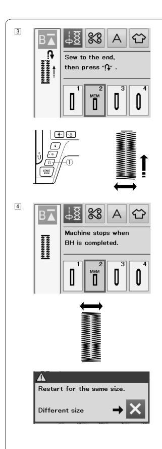
3 Start sewing again, and the machine sews the front bartack and right side of the buttonhole. Stop the machine when you reach the ending point. Then press the reverse button ①.
