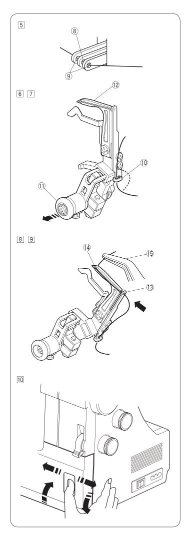
5 Turn the handwheel toward you several times to align the eye of the looper take-up lever and both guide holes.
